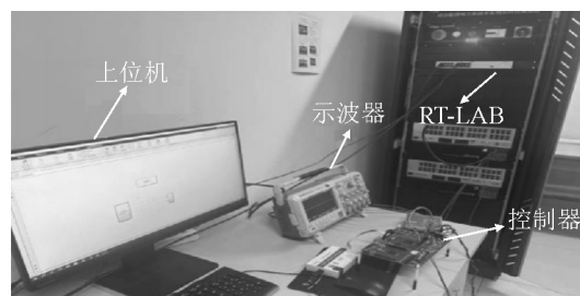
图11 RT-LAB半实物实验平台 Fig. 11 RT-LAB hardware-in-the-loop (HIL) experimental platform
